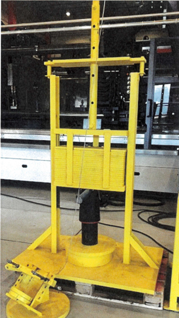
Picture 3. Axial testing with PIN protector.
