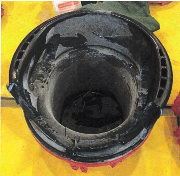
Picture 21. BOX protector after angular impact. -46 °C.
