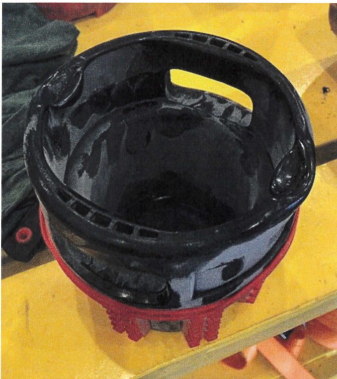
Picture 16. BOX protector after axial impact. -46 °C.
