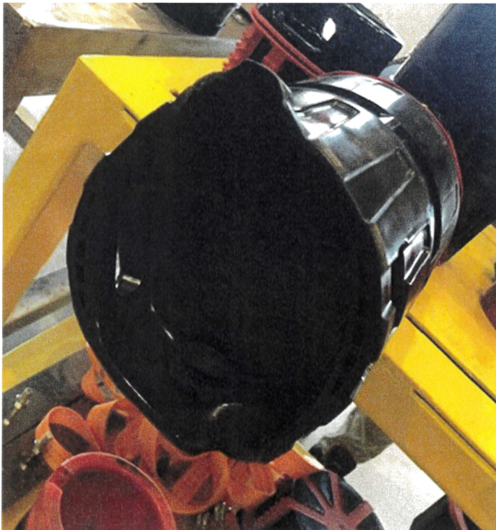
Picture 8. PIN protector after axial impact. 21 °C.
