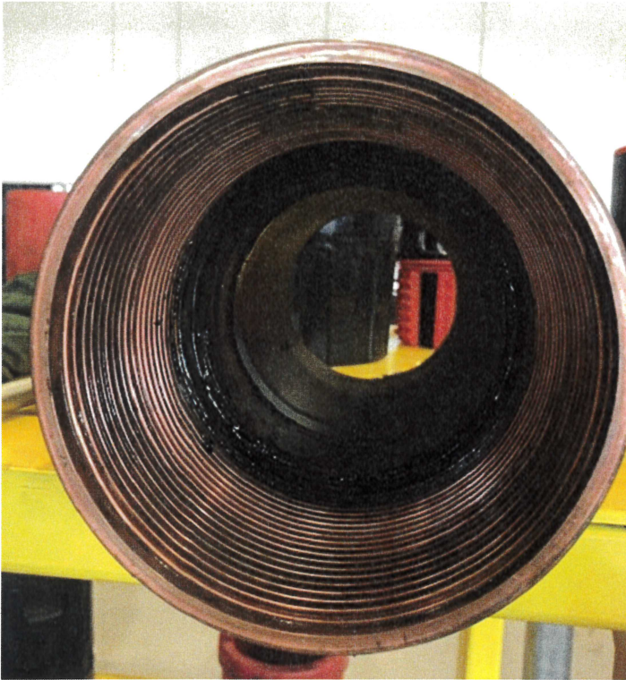
Picture 17. After testing. No damages.
