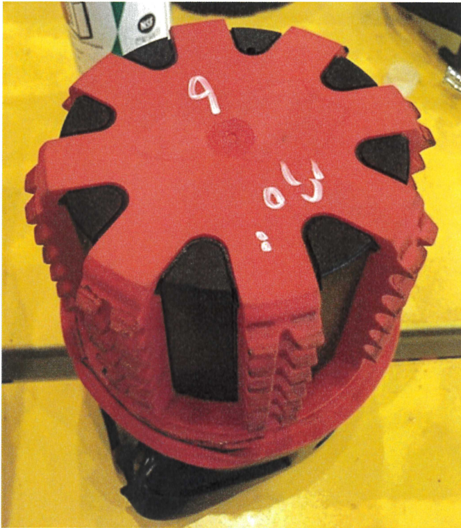
Picture 15. BOX protector after axial testing.
