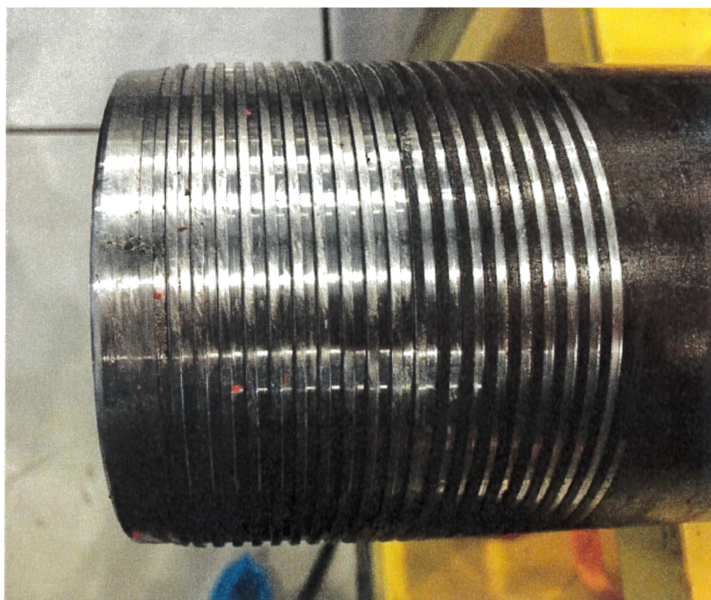
Picture 12. After testing. No damages.
