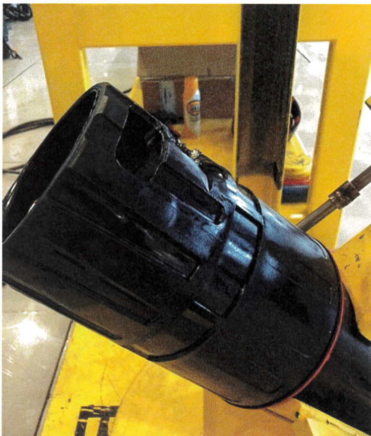
Picture 18. PIN protector after angular impact. 21 °C
