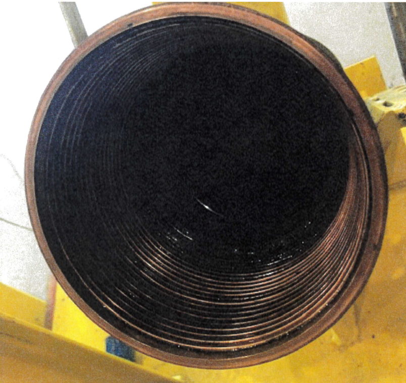
Picture 23. After testing. No damages or ovality.
