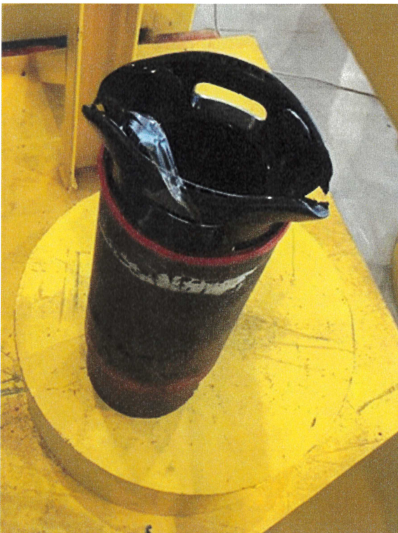
Picture 14. BOX protector after axial impact. 66 °C.
