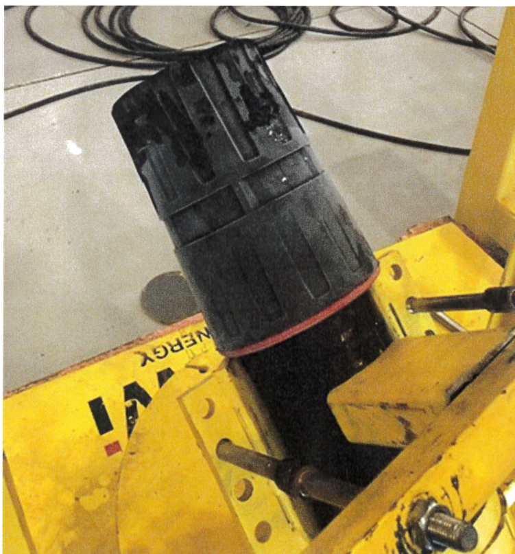
Picture 19. PIN protector after angular impact. -46 °C.
