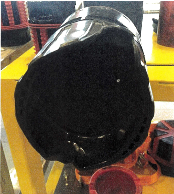
Picture 9. PIN protector after axial impact. 66 °C.
