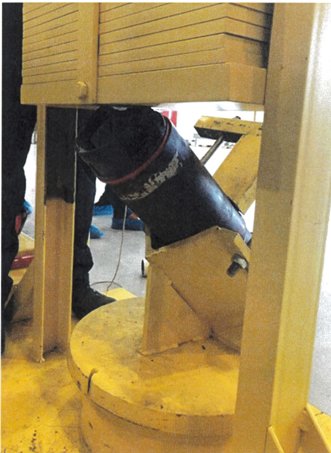
Picture 5. Angular testing with BOX protector.
