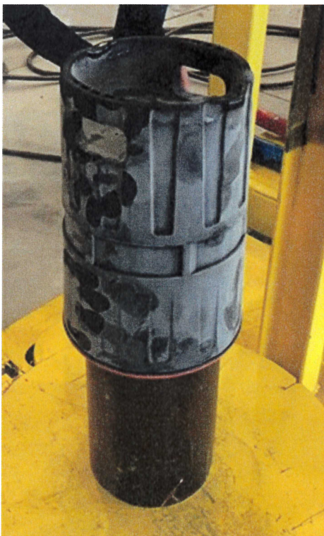
Picture 10. PIN protector after axial impact. -46 °C.
